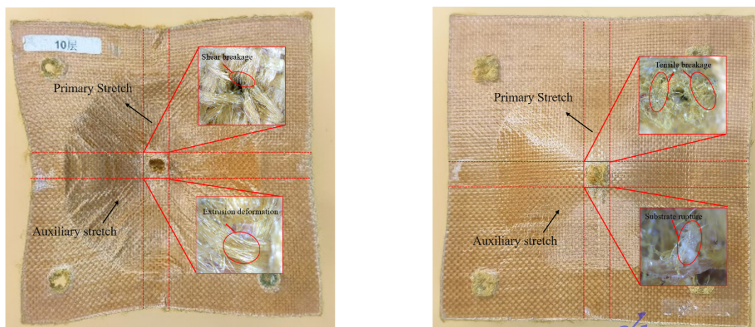
(a) Failure morphology of the PBO fiber composite laminate (front side)
